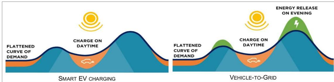
Figure 6 - Smart EV charging and V2G scheme (Corchero Garcia, 2022).
