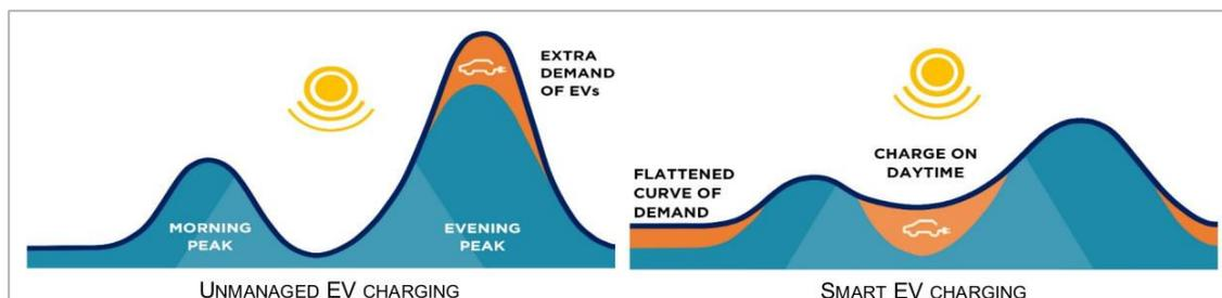
Figure 3 - Unmanaged EV charging and smart EV charging scheme (Corchero Garcia, 2022).
