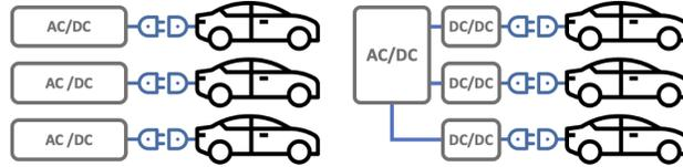
Figure 1: Single-port chargers (SPCs) on the left, and multi-port chargers (MPCs) on the right.
